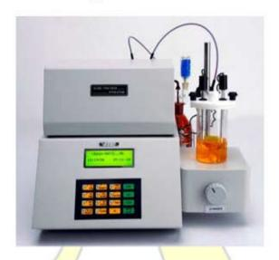
The model MATIC – MD is Micro-Controller Based Automatic Karl Fischer Titrator designed for accurate estimation of moisture contents in various samples. It is used in QA, QC and R&D labs in Pharmaceutical, Chemical and other industries.
